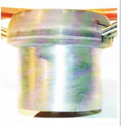
For ease of handling, glue the lower hub section to the sleeve first. Apply J-B Weld to the inside diameter and the sleeve, making sure there is enough to fill the cavity between them.
