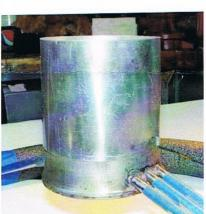
Push the sleeve on the cup to test the fit and set up the fixturing to press it. Take it apart and apply the great "slow setting" J-B Weld glue (or an equivalent two-part epoxy non-running glue) to the cup and sleeve contact areas.
