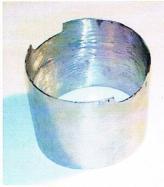
After squarely cutting the 3" aluminum tube, rough sand the inside so glue will stick and finely sand the outside until it's smooth.
