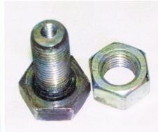
Drill 0.1590" holes 0.9" deep into the end of three 7/16"—20 x 1" screws. Tap the holes for the #10x32 horn ring screws.
