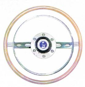
Here is another idea. This method could be used to build a wheel that combines the harp-spoke with a modern hub like this.
