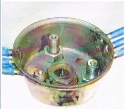
Install the three horn screws in the round holes of the wheel cup. Through trial and error, make sure they align with the holes in the horn ring. The heads of the bolts may need grinding and the holes filed to get the bolts installed in the proper position.
