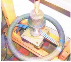
some large clamps may also work for this process. The top edge of the sleeve will expand as it is pressed. Stop when the cutouts touch the spokes. A slight splitting at the cutout radii is acceptable.
