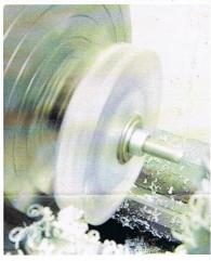
Machine the upper and lower hub sections according to the drawing. Plexiglas makes a very good material because it is stable, easy to machine and glues very well with Acrylic Glue (Methylene Chloride). Test some sample glue joints first to make sure you are using the right glue for the plastic.
